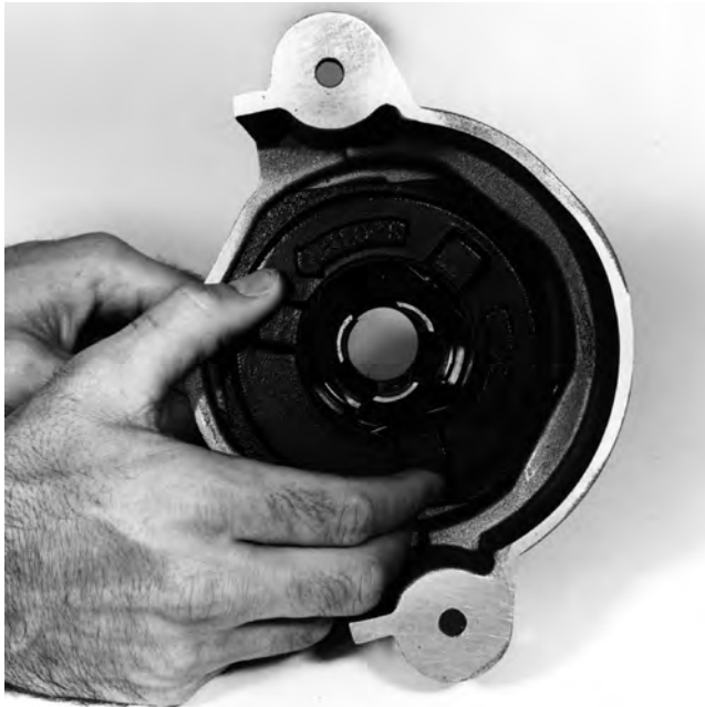
Figure 12 – Remove Jaw Set Cover
