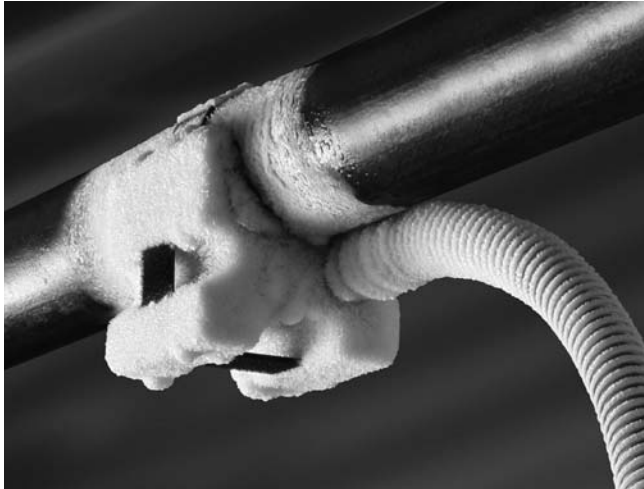
Figure 9 – Freeze Head Frozen to Pipe
