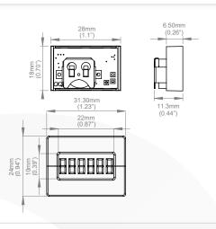
Miniature, 6 digit LCD totalising counter suitable for either direct PCB mounting, or panel mounting with bezel supplied.
