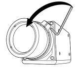
2. Focus the camera by rotating the lens.
