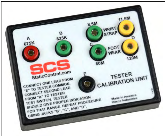
Figure 13. SCS 770033 Calibration Unit
