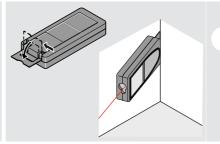
I he orientation of the endpiece is automatically detected and the zero point is accordingly adjusted.
