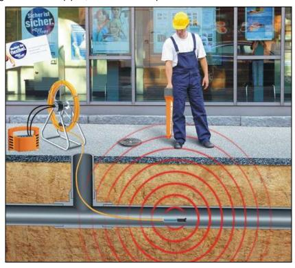
Alternatively, any other active probe (e.g. a camera probe) with adequate transmitting frequency (see Technical Data) can be located using the receiver. For a detailed description, please refer to the manual of the respective product.
