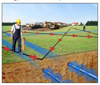
Carry out a passive survey in **POWER GRID** and **RADIO** modes using a grid search pattern to cover the site and locate conductors in all directions.
