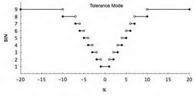
Figure 3.18 – Bin Setup Tolerance Mode Graph
