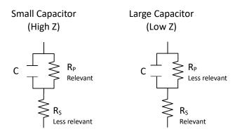
Figure 3.8 – Equivalent Capacitor Circuit
