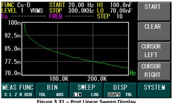
Figure 3.31 – Post Linear Sweep Display
