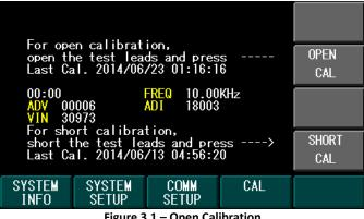
Figure 3.1 – Open Calibration
