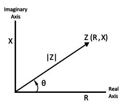
Figure 3.6 – Complex Impedance Plane
