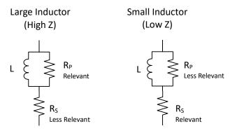
Figure 3.9 – Equivalent Inductor Circuit
