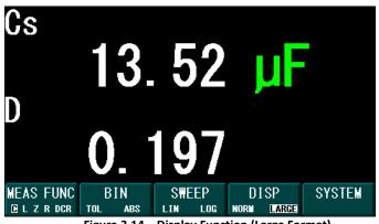
Figure 3.14 – Display Function (Large Format)
