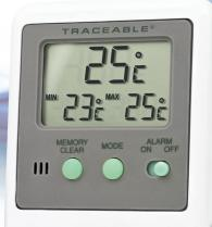
View MIN/MAX readings and set alarms to monitor temperature sensitive materials over any time period
