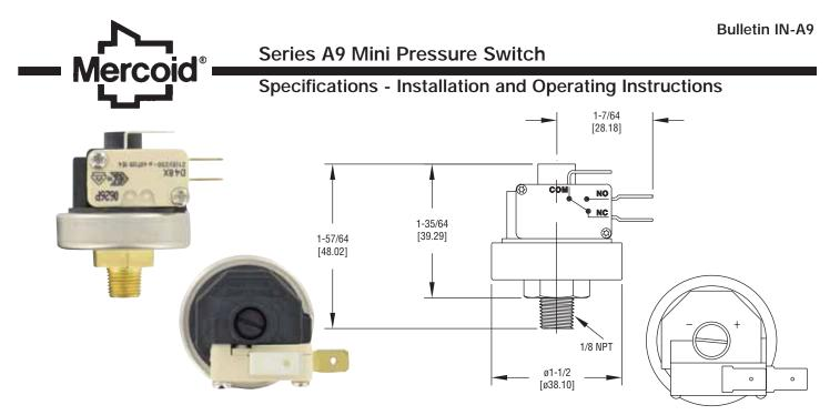
**Series A9 Pressure Switches** are designed for controlling pressure with higher current capacity. These switches are used widely in steam cleaners, steam irons, and other pressure control systems. It provides SPDT contact and Series A9 Pressure Switches utilize high-quality miniature snap-action switches. The switch is diaphragm operated, boasting a high temperature rating and compact size.
