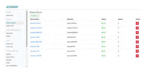
A device that is successfully connected and communicating with the gateway will have a green 'ON' mark under the status column. Whiles a device that is offline will display a red 'OFF' warning symbol.
