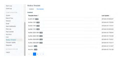
To upload a new device template click on the 'New/Update' tab. All Accuency device templates can be found in the remote update section of the page. In order to use the remote upload function, users must ensure they have sufficient connection to the Internet.
