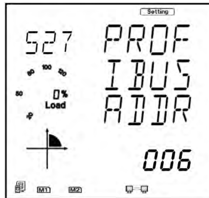
Figure 5-50 AXM-PROFI address setting on meter display
