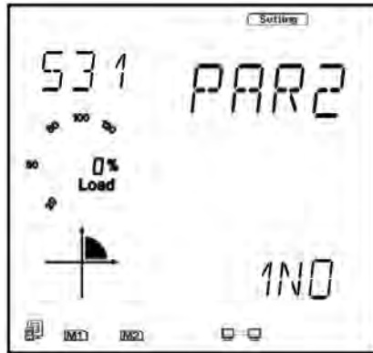
Figure 5-54 Parity setting for the AXM-RS485 module
