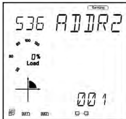
Figure 5-55 Address setting for AXM-RS485
