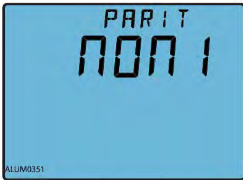
Fig.3-57 Extend IO communication check setting
