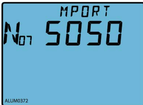
Fig.3-79 MODBUS-TCP port setting
