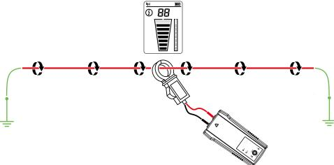
Figure 4.12a: Connecting the clamp
