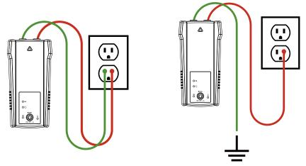
Figure 3.2a: Simplified direct connection
