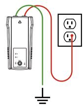
Figure 3.1a: Proper connection with separate ground
