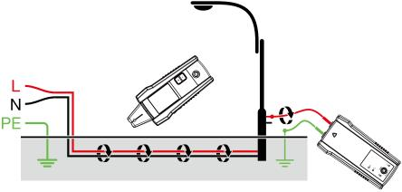
Figure 4.7: Tracing underground wires
