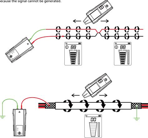
Figure 2.2a: Generating a signal with HIGH mode
