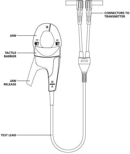
Figure 2.3: Overview of CT-400 Signal Clamp
