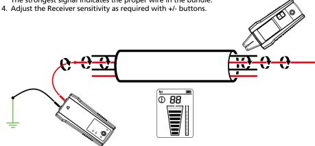
Figure 4.9: Identifying a specific wire in a bundle
