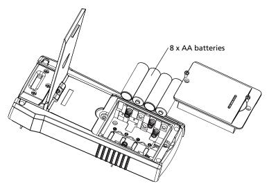
Figure 5.1a: Changing the Transmitter batteries
