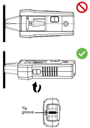
Figure 3.1d: Aligning the Tip Sensor groove
