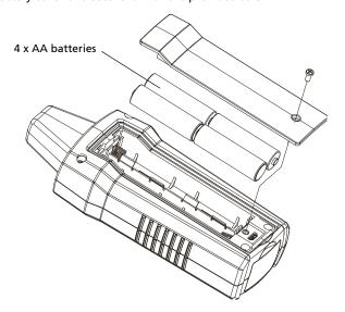
Figure 5.1b: Changing the Receiver batteries
