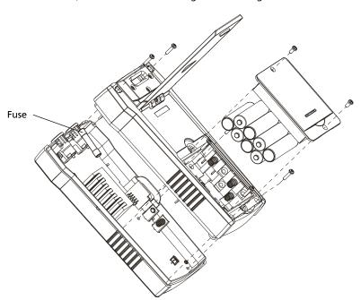
Figure 5.2: Transmitter fuse replacement
