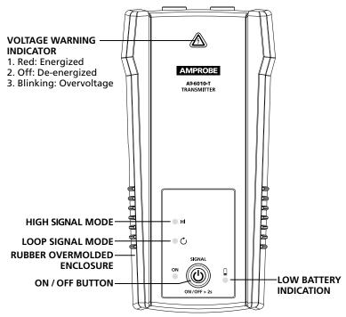
Figure 2.2c: Overview of AT-6010-T Transmitter
