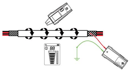
Figure 4.6b: Tracing a shielded wire disconnected from the ground at far-end
