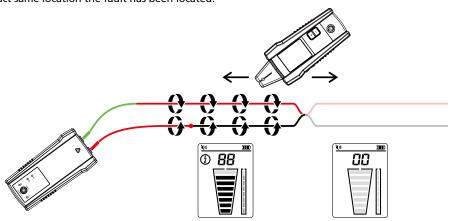
Figure 4.3: Tracing a cable to find shorts
