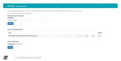
Users can click on 'Detail' to view the description of the configuration file. The details include the Model name, serial number, time created. firmware version and the description entered when the backup was created.
