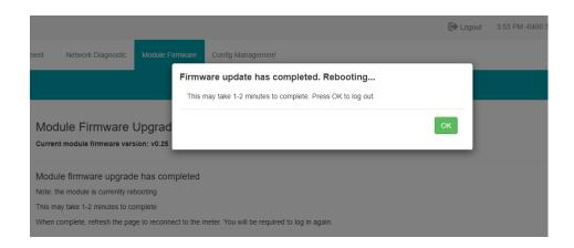
After the module reboots, users will be able to log back into the web interface. When logged in click on the 'About' tab located on the top right corner of the web page to view the 'Device Information' page. From the Device Information page users can ensure that the meter was updated correctly to the right firmware version.
