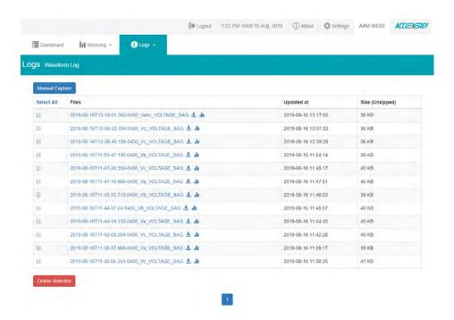
To view the waveform click on the icon. Users can select which voltage or current phase they want to view on the graph during the power quality event.
