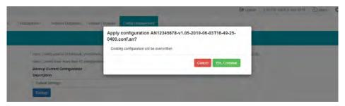
A module reboot is required for the configuration to take effect. if users decided to reboot later the reboot must be performed from the Management page in order for the settings to take effect on the device.
