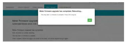
After the meter reboots, users will be able to log back into the web interface. When logged in click on the 'About' tab located on the top right corner of the web page to view the 'Device Information' page. From the Device Information page users can ensure that the meter was updated correctly to the right firmware version.
