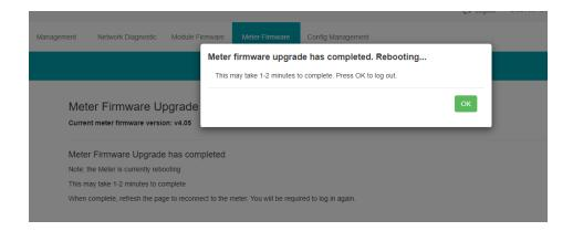
After the meter reboots, users will be able to log back into the web interface. When logged in click on the 'About' tab located on the top right corner of the web page to view the 'Device Information' page. From the Device Information page users can ensure that the meter was updated correctly to the right firmware version.
