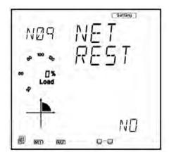
Press 'P' to get to "N10 PASSREST". Press 'V/A' to configure the password reset. The cursor
