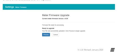
After the firmware has uploaded to the web server, click on 'Process'.
