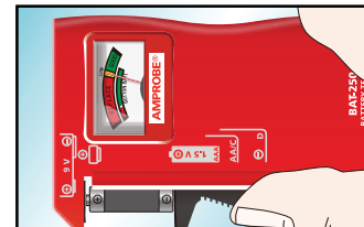
Testing 1.5 V battery (AAA, AA, C, D)
