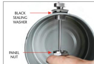
5. Place the black sealing washer over the probe tip and insert through the 9/16 inch diameter hole of the container from the outside. Place the panel nut over the end of the probe tip as shown from the inside of the container and thread the two pieces together.
