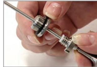
3. Insert data logger probe tip through the receptacle.
