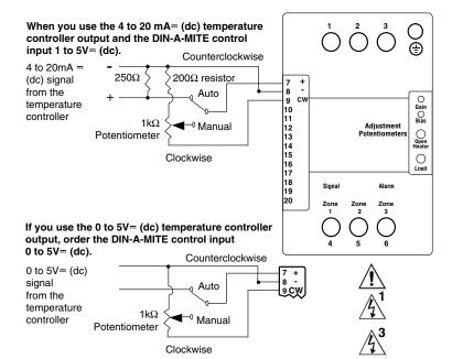
NOTE: The potentiometer and resistors are customersupplied. For the potentiometer control assembly only, order Watlow part number 08-5362.
