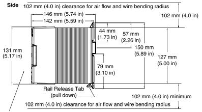
Front panel is touch-safe, no clearance is required.
