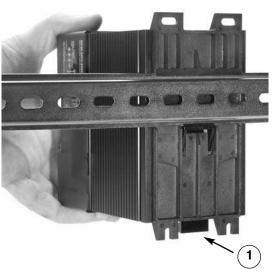
1. Press down on the release tab while rotating the unit up and away from the rail.
