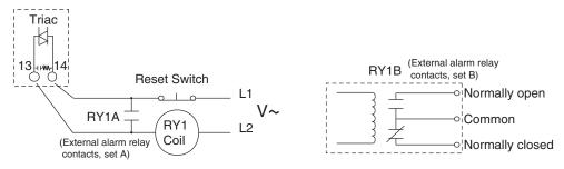
**Latching Alarm Relay Circuit**
