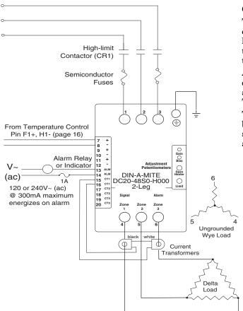
Non-latching Alarm Option (models DC\_\_-\_S\_-H\_\_\_)
