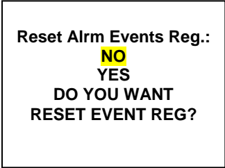
Figure 36: Resetting Alarm Events Register
