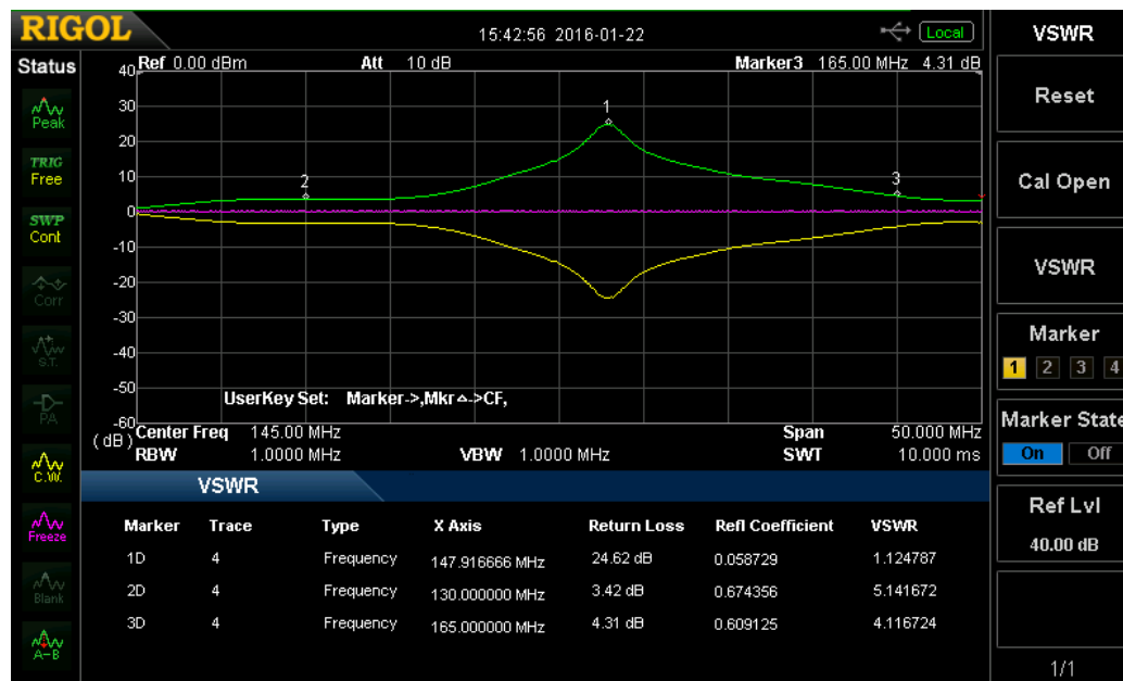
Figure 2-12 VSWR Measurement Interface
