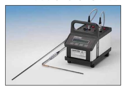
Wherever there is a demand for reliable and accurate temperature measurement, you can rely on the JOFRA DTI-1000 reference thermometer and the JOFRA STS reference probes; backed on more than 50 years of experience.
