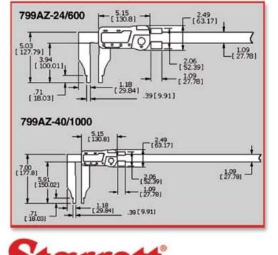
0-40"/ 1000mm Extended Range Electronic Caliper
