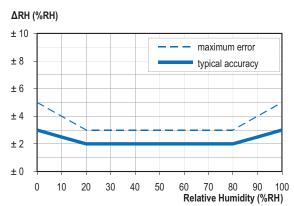
Typical accuracy of relative humidity measurements given in %RH for temperatures 0 to 80°C.
