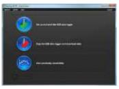
Click on the 'Set up and start the USB data logger' button.
