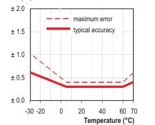
SENSOR ACCURACY & INFORMATION Typical and maximal tolerance for temperature sensor in °C.
