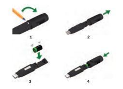
EL-USB-1 PRO Before using the data logger you will need to insert the 3.6V 2/3AA High Temperature battery provided, following the instructions below.
