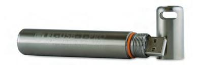
This standalone data logger measures and stores more than 32,000 temperature readings over a -40 to +125°C (-40 to +257°F) range with a resolution of 0.1°C (0.2°F).
