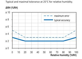
Typical accuracy of relative humidity measurements given in %RH for temperatures 0 to  $80^{\circ}\text{C}$ .
