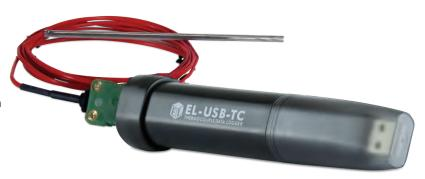
This standalone data logger measures and stores more than 32,000 temperature readings from a J, K or T-type thermocouple at a resolution of  $0.5^{\circ}$ C (1°F). It comes supplied with a K-type thermocouple capable of measuring from 0 to +200°C (+32 to +392°F).
