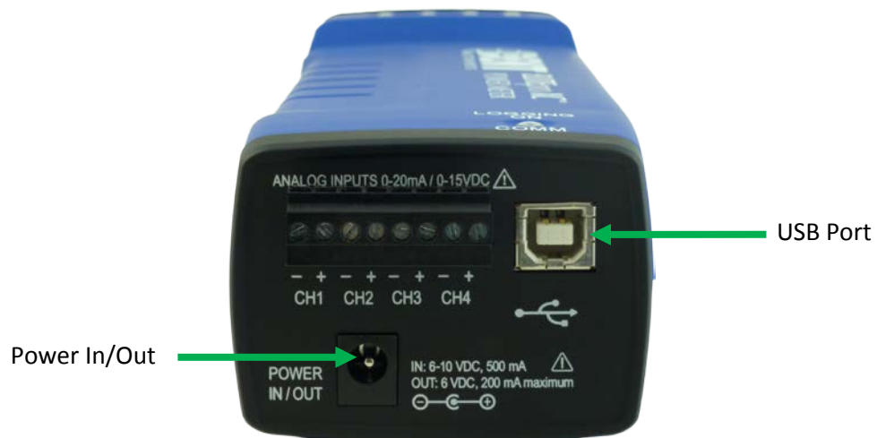
Power End Panel Connections
