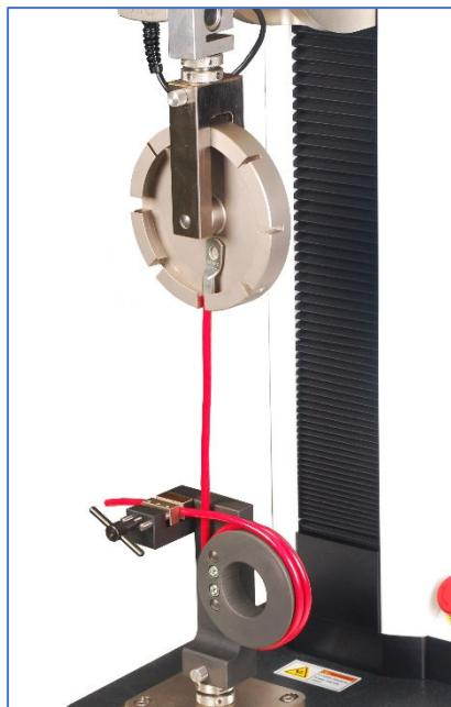
A wire crimp pull test determines how much force is required to remove the terminal. For durability analysis, force measurement systems can also pull to a specified load and hold the load for a given period.
