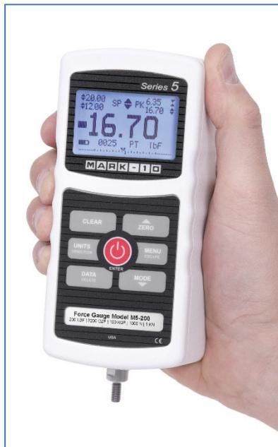
The ubiquitous force gauge is an instrument which may be hand-held or mounted to a fixture or test stand. It contains an internal load cell, with electronics and a display. A threaded shaft is commonly affixed to the load cell, and protrudes from the housing of the instrument. Grips, fixtures, and implements to engage the sample may be mounted to the shaft.
