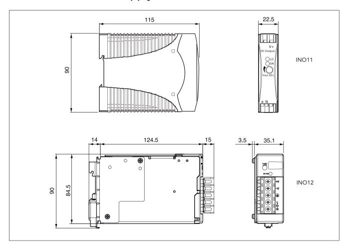
The power supply units in the Intellinova system are intended for mounting on standard DIN rail. INO11 is used to supply a standard Intellinova System Unit with a power consumption of max. 18 W.
