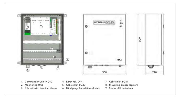
The Intellinova System Unit INS10 is comprised of an industrial enclosure, a Commander Unit, internal cabling and terminals for power supply. Up to four monitoring units can be mounted and are ordered separately. The enclosure, intended for wall mounting, is robust and sealed for use in harsh environments.
