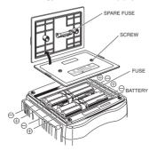
▲ CAUTION Install batteries in correct polarity as marked inside.
