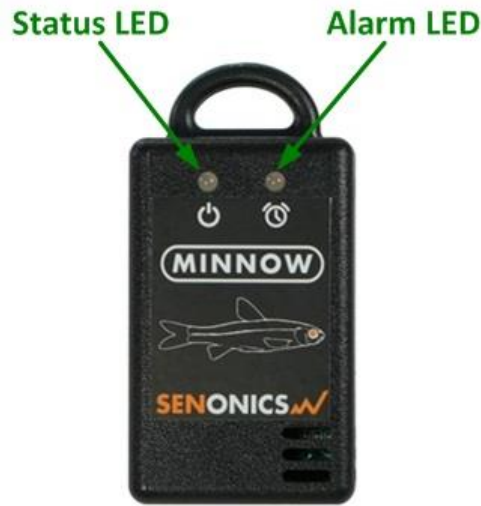
Figure 2: Minnow Alarm Indicators
