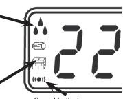
Sound Indicator (Press and hold the Lock/Beep Button for 3 seconds to turn on/off. Beep will sound faster the higher the moisture content.)
