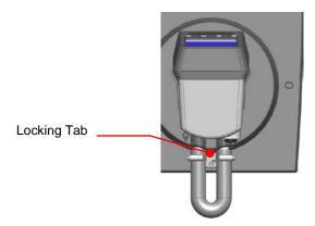
2. Rotate the Temperature Controller clockwise until it stops (about 0.75 inch / 1.9 cm).
