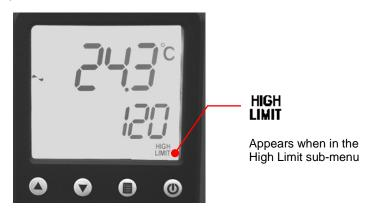
To Access: Press the key until HIGH LIMIT appears on the display.
