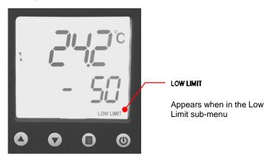
**To Access:** Press the key until LOW LIMIT appears on the display.
