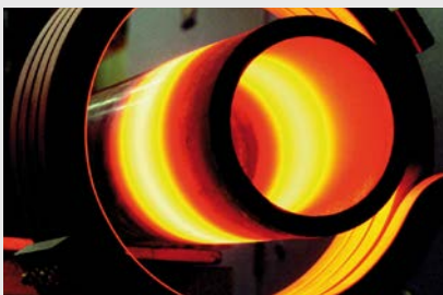
Inductively heated pipe
