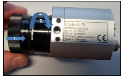
Figure 13: Inserting the lens
