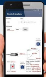
The measuring spot size of the respective device is calculated for each distance
