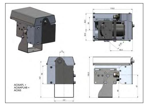
**Figure 20:** Air purge (ACXIAPL) with mounting bracket (ACXIAPLAB) and shutter (ACXIS), dimensions [mm]
