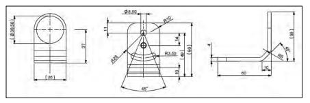
**Figure 4:** Mounting bracket, adjustable in one axis, with tripod thread **[Order No. - ACXIFB]** – standard scope of supply
