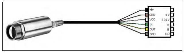
Figure 24: Configuration terminal block Xi 80/410
