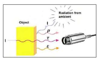
Figure 50: Composition of IR radiation
