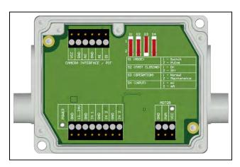
Figure 43: Control box Shutter
