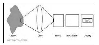
Figure 48: Main principle of non-contact thermometry
