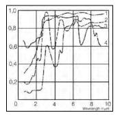
Figure 51: Spectral emissivity of several materials: 1 Enamel, 2 Plaster, 3 Concrete, 4 Chamotte
