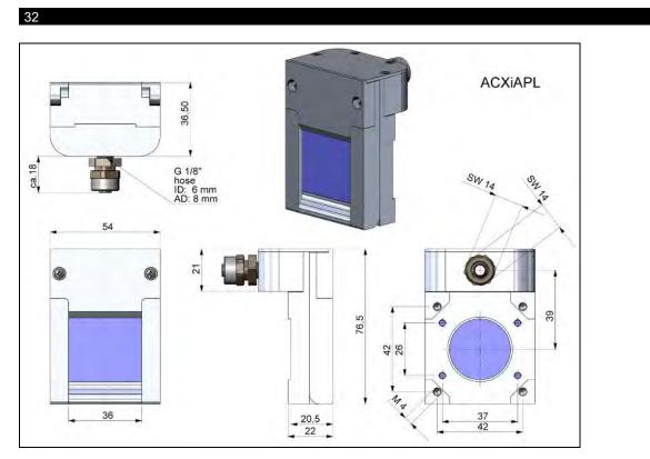
Figure 9: Laminar air purge with Si protective window, dimensions [mm]
