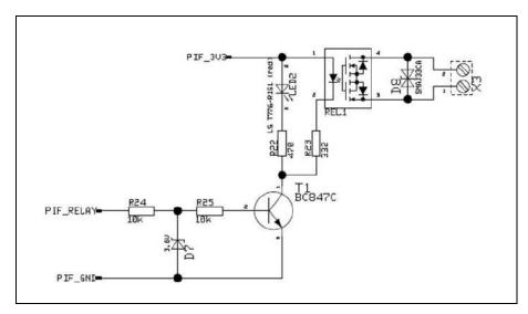
Figure 58: Relay output at industrial PIF
