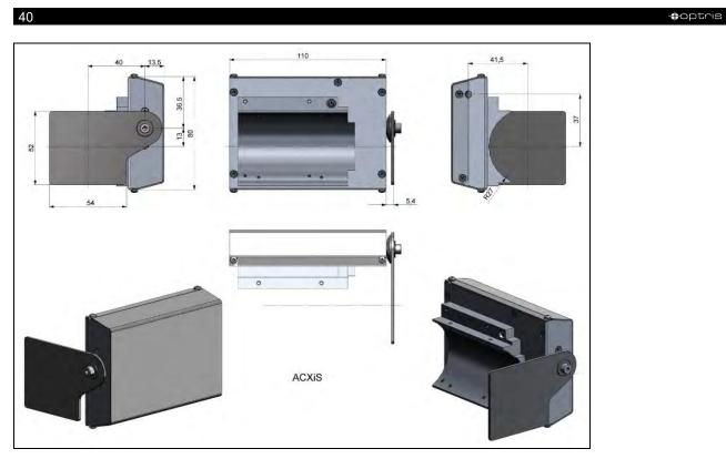
Figure 15: Shutter (ACXIS), dimensions [mm], weight: 550 g
