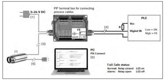
Figure 32: Fail-Safe monitoring states
