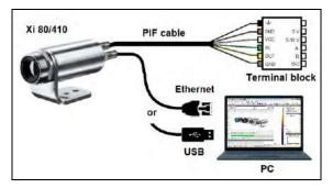
**Figure 36:** Connection Xi 80/410 to PC via Ethernet/USB
