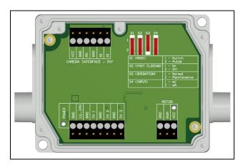
Figure 43: Control box Shutter
