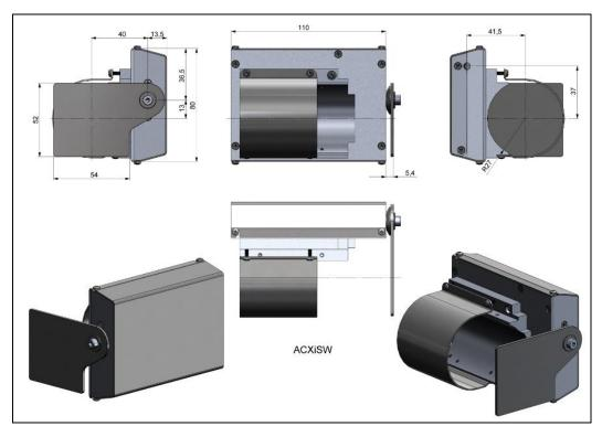
Figure 13: Shutter for water cooling (ACXISW), dimensions [mm], weight: 600 g
