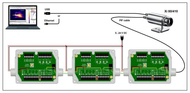
Figure 30: Connection of 3 industrial PIFs via RS485
