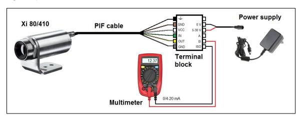
Figure 40: Electrical installation for autonomous operation Xi 80/410
