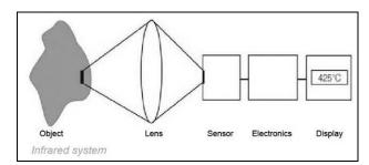
Figure 48: Main principle of non-contact thermometry
