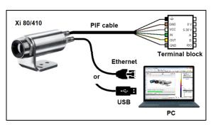
**Figure 36:** Connection Xi 80/410 to PC via Ethernet/USB
