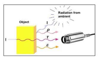
Figure 50: Composition of IR radiation
