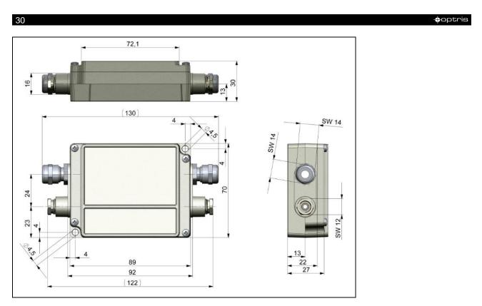
Figure 8: Industrial/stackable PIF (Process Interface) – electronic box, control box shutter, dimensions [mm]
