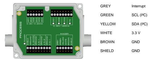
Figure 31: Connections of the industrial Process Interface for Xi 400
