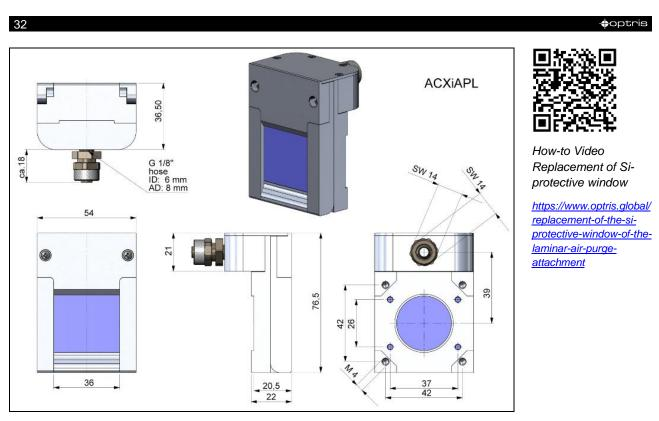
Figure 9: Laminar air purge with Si protective window, dimensions [mm]
