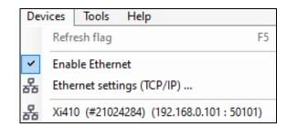
To change the address settings, go to **Devices** and **Ethernet settings (TCP/IP)**. The address for the device is assigned under **Device address**. This must have a different address (last block) to the other participant (e.g., PC) (**Send to address (local computer)**). It is important that the network part (first three blocks) must be identical for both addresses. The address range of the individual blocks can be between 0 and 255.
