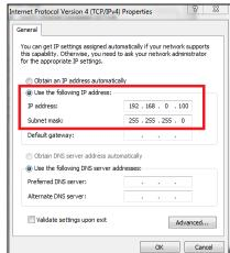
In the register card **General** enable the checkbox **Use the following IP address**. Now enter a user defined IP address for your PC (192.168.0.100). This must be identical to the address set in the PIX Connect software.
