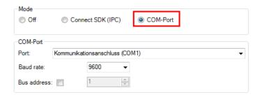
3. Select the baud rate that matches the baud rate of the other communication device. The other interface parameters are 8 data bits, no parity and one stop bit (8N1).
