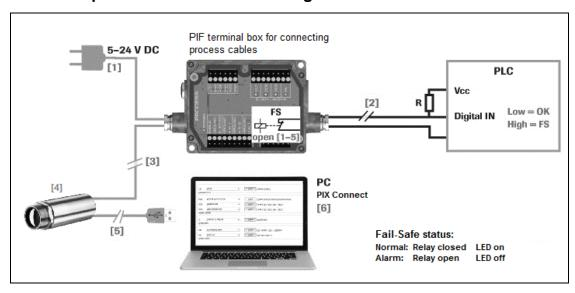
Figure 32: Fail-Safe monitoring states
