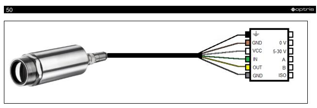
Figure 24: Configuration terminal block Xi 80/410
