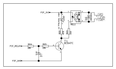
Figure 58: Relay output at industrial PIF
