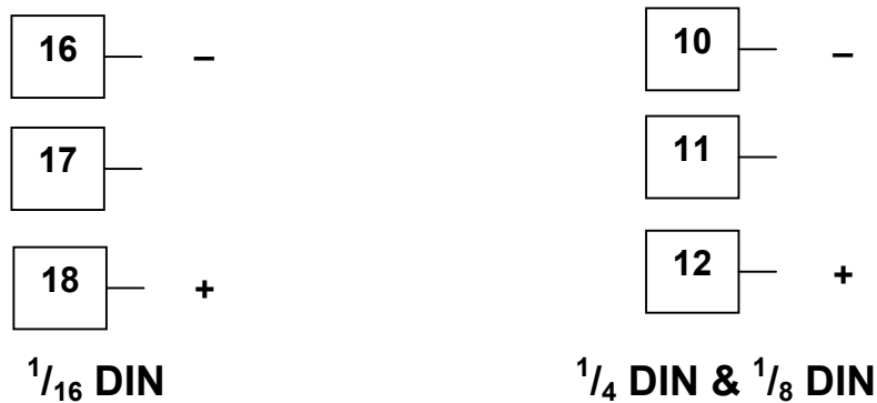
Figure 28. Option Slot 3 - SSR Driver Module
