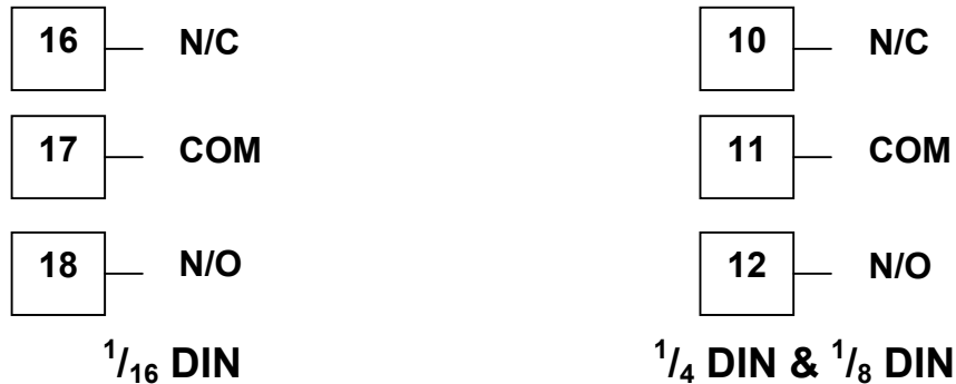
Figure 27. Option Slot 3 - Relay Module
