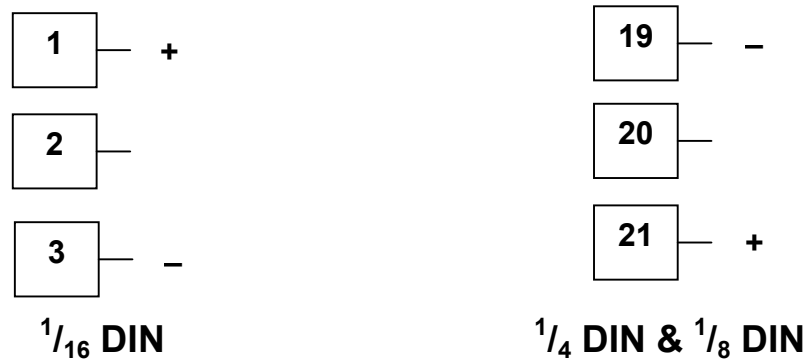
Figure 21. Option Slot 1 - Linear Voltage & mADC Module
