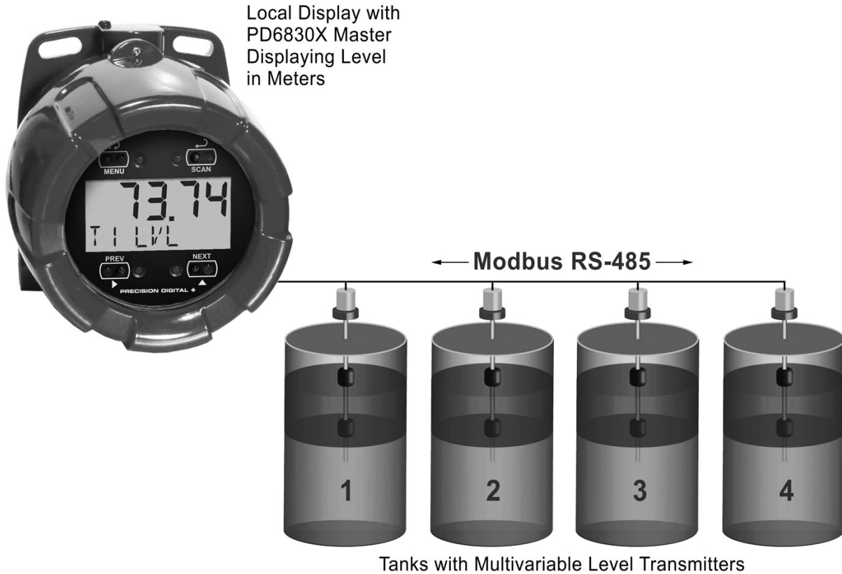
Example 1 Level Transmitter Setup, Register Numbers, & Process Variables
