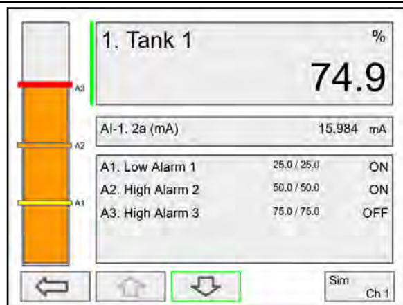
The bargraph changes to orange above set point 2
