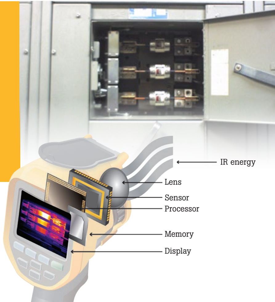
Figure 1. Anatomy of an infrared camera
