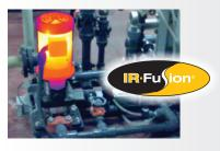
The 3.5" LCD touchscreen offers IR-Fusion™ to blend a visible light image with an infrared image to more easily locate problems. Simply slide your finger across the screen to adjust the setting.
