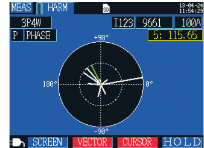
Harmonic power phase angle graph screen
