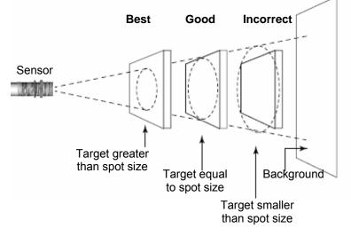
Figure 2: Proper Sensor Placement
