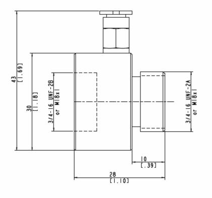
Figure 9: Dimensions of Air Purge Collar
