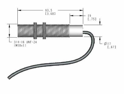
Figure 3: Dimensions of sensor
