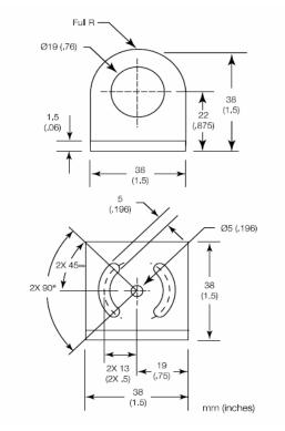
Figure 7: Dimensions of Fixed Mounting Bracket
