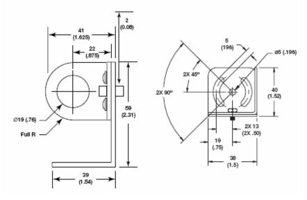
Figure 8: Dimensions of Adjustable Mounting Bracket
