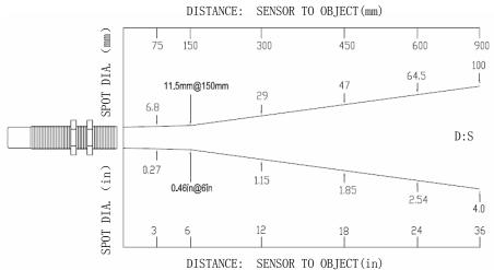
Figure 1: How to read the optical diagram
