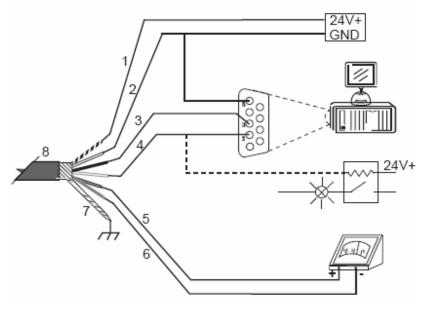
Figure 5: connection diagram
