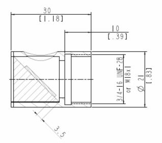
Figure10: Dimension of Right Angle Mirror
