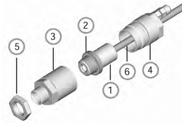
Figure 58: Mounting the Air Purge Jacket
