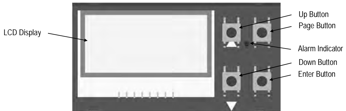
Figure 33: Control Panel for the Comm Box (DIN)
